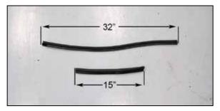
11. Cut the provided edge trim into two sections, one section is to be 32" long and the other section is to be cut at 15" long.
