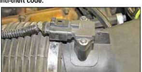
2. Disconnect the inlet air temperature sensor electrical connection.
