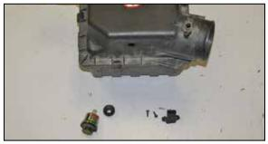
17. Remove the inlet air temperature sensor. On vehicles equipped with a filter minder, remove the filter minder and grommet from the air box.
