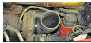
16. Install the provided 90° hose onto the turbo inlet and secure with the provided hose clamps. NOTE: Do not completely tighten the hose clamp at this time.
