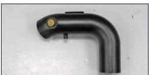
19. On vehicles equipped with a filter minder, install the factory filter minder grommet and filter minder into the K&N intake tube as shown. On vehicles that are not equipped with a filter minder, install the provided plug into the K&N intake tube.
