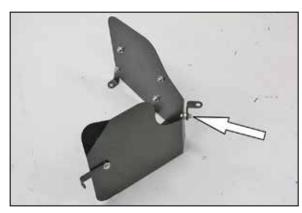
10. Install the tube mounting bracket (070712) onto the heat shield using the provided spacer and hardware as shown.
